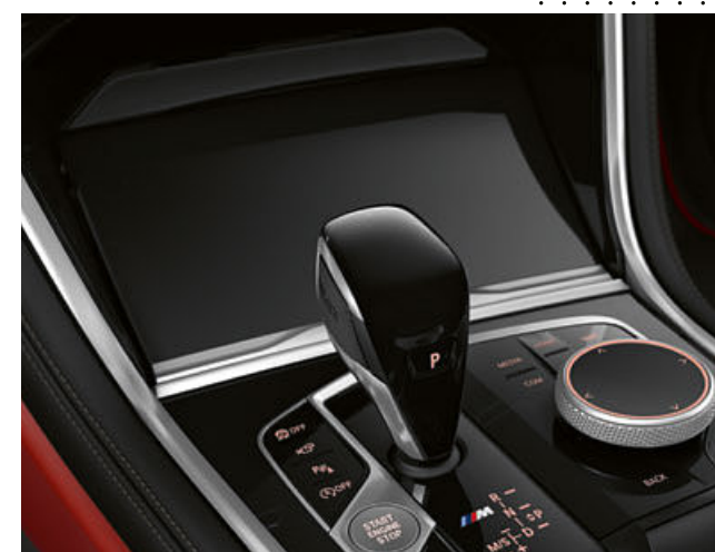
Breathtaking Black: The complex, multi-stage production process begins with the application of several layers of dyed tulip wood. The special intensity of the surface is created during the finishing process by repeatedly applying and polishing deep black piano finish. The result is an incredible colour depth.
